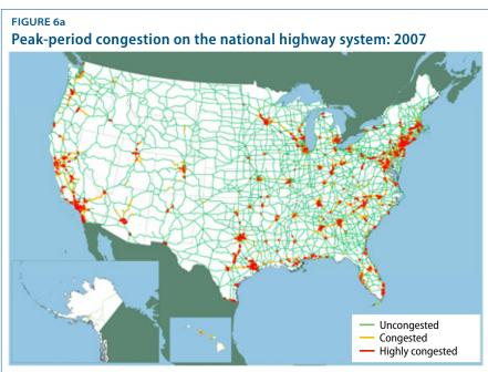
Note: Highly congested segments are stop-and-go conditions with volume/service flow ratios greater than 0.95. Congested segments have reduced traffic speeds with volume/service flow ratios between 0.75 and 0.95. The volume/service flow ratio is estimated using the procedures outlined in the Highway Performance Monitoring System Field Manual, Appendix N.
